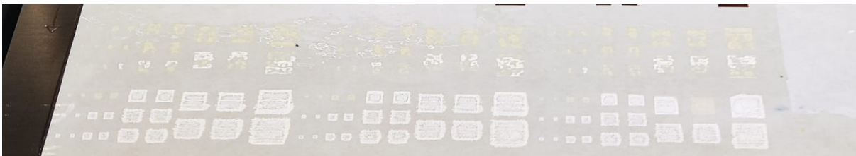
Figure 19: Inkjet printed Cs 3 Cu 2 I 5 layer on PI flexible substrate. Pattern of squares ranging from 1 mm 2 to 1 cm 2 .
