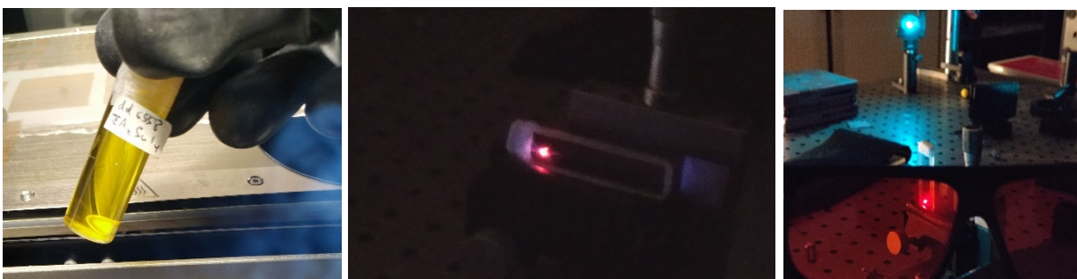
Figure 33. Ink bottle and PL colour under laser of 488nm of \text{TEA}_2\text{SnI}_4 inkjet printed layers into glovebox, inert conditions ( \text{N}_2 ).
