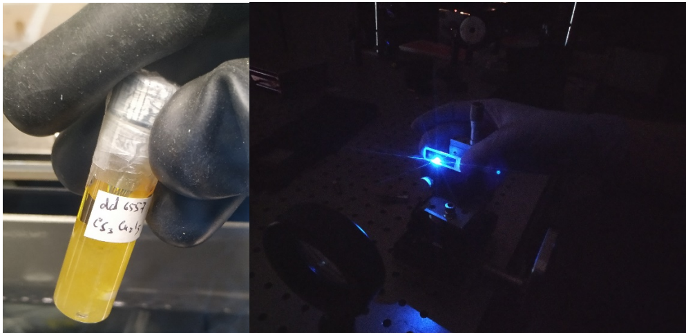
Figure 18: Cs 3 Cu 2 I 5 inkjet printed layers into glovebox, inert conditions (N 2 ). Ink bottle and PL colour under laser of 488nm.
