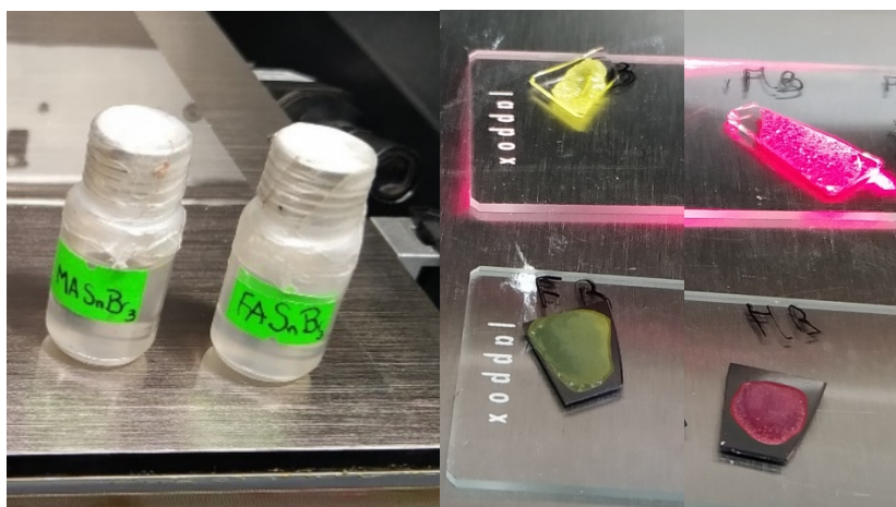
Figure 9. \text{FASnBr}_3 , \text{MASnBr}_3 inkjet printed layers into glovebox, inert conditions ( \text{N}_2 ). Ink bottles and optical photo with expected colors for each ink onto silicon and fused silica for PL (under laser of 488nm) and TRA measurements, respectively.
