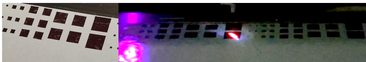
Figure 34. Inkjet printed \text{TEA}_2\text{SnI}_4 layer on PI flexible substrate emitting in the red range under UV pointer excitation. Pattern of squares ranging from 1 \text{ mm}^2 to 1 \text{ cm}^2 .
