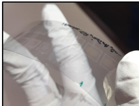
Figure 9. Picture of SnO 2 layers printed on PET/ITO substrate showcasing their flexibility and transparency.
