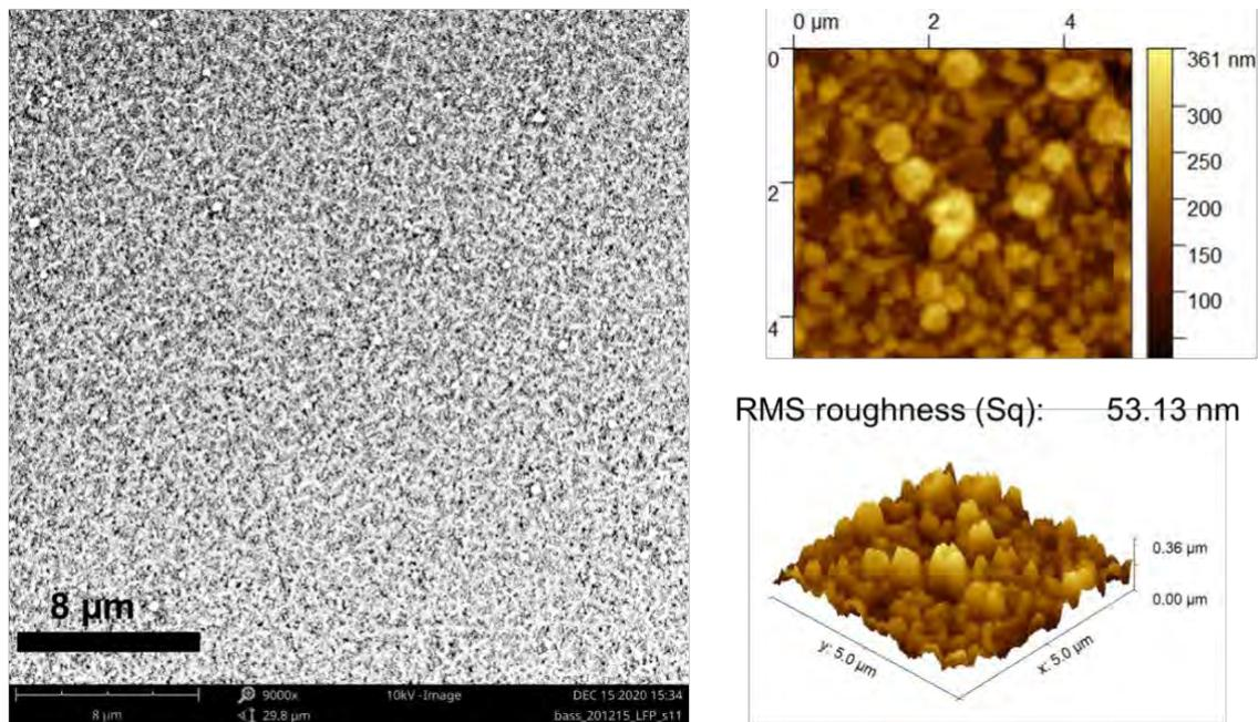
**Figure 4.** (left) SEM image of inkjet printed  $\text{Ag}_3\text{BiI}_6$  thin film. (right) 2D and 3D AFM topography images of printed  $\text{Ag}_3\text{BiI}_6$  thin film.
