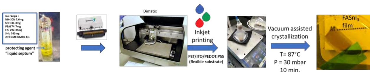
**Figure 1.** Schematic of individual steps involved in inkjet printing of FASnI<sub>3</sub> thin films in ambient environment.
