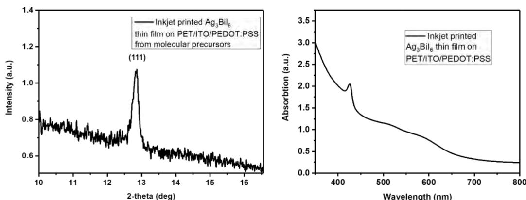
**Figure 4.** (left) XRD pattern of inkjet printed  $\text{Ag}_3\text{BiI}_6$  thin film on flexible PET/ITO/PEDOT:PSS substrate. (right) absorption spectrum of  $\text{Ag}_3\text{BiI}_6$  thin film on flexible PET/ITO/PEDOT:PSS substrate.
