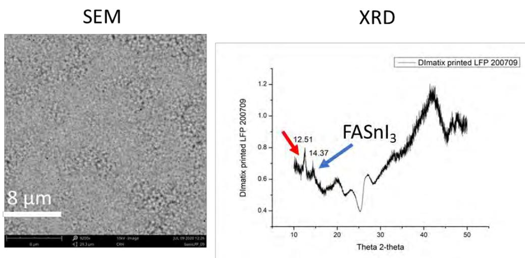
**Figure 2.** Inkjet printed  $\text{FASnI}_3$  thin film in ambient conditions and crystallized using vacuum assisted annealing process on a flexible PET/ITO/PEDOT:PSS substrate: (left) SEM image and (right) XRD pattern. Blue arrow indicates the diffraction peak of the (100) plane for  $\text{FASnI}_3$ , while the red arrow indicates the signal from some byproduct.
