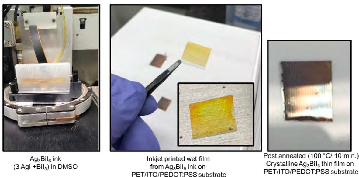
**Figure 3** (left)  $\text{Ag}_3\text{BiI}_6$  precursor ink filled into DIMATIX cartridge. (middle) Inkjet printed wet film from  $\text{Ag}_3\text{BiI}_6$  precursor ink on PET/ITO/PEDOT:PSS substrate.
