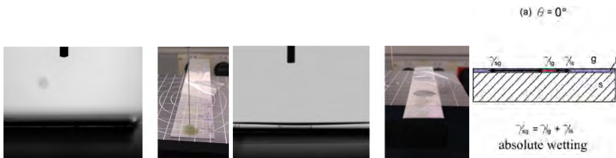
Figure 5: Complete wettability by contact angle of \sim 0^\circ . Left, \text{Cs}_2\text{SnI}_6 ink on PET. Right, HTL PEDOT:PSS ink on PEN.
