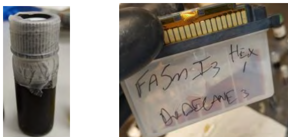
Figure 15: Preparation of ink and printhead into the glovebox of \text{FASnI}_3 based on hexane+dodecane.
