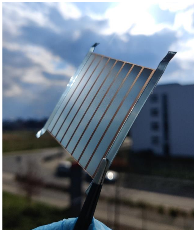
Figure 1. 8-cell interconnected flexible large area lead-free perovskite ( \text{Dip}_2\text{FA}_9\text{Sn}_{10}\text{I}_{31} ) solar module.
